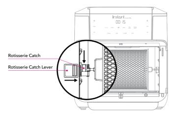
3. Align the left side of the accessory with the hole in the rotisserie catch, and set the right end of the accessory in the notch on the right.
