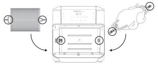
2. Move the red rotisserie catch lever to the right and hold it in position. Notice that the rotisserie catch inside the cooking chamber withdraws slightly when you move the lever.
